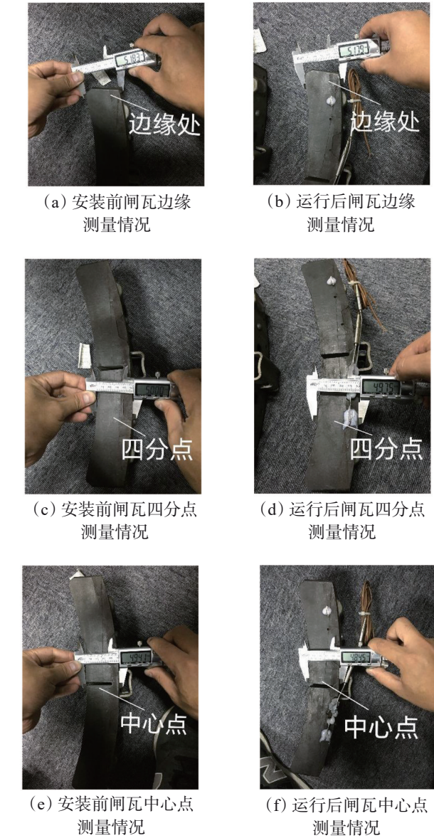
图 16 闸瓦磨耗运行前后测量情况 Fig. 16 Measurements of brake shoe wear before and after operation
